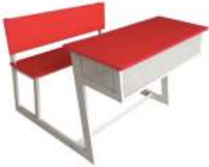
ADELMO (Grade IX & above) Size : 1200W 400D 450-750H CRC powder coated structure with PLCB seat, back & table top Option : Grade I to IV / Grade V to VIII
